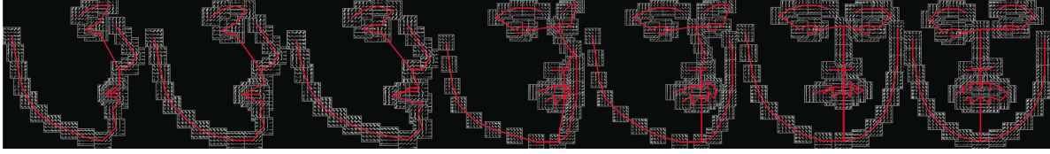
Figure 2.3: The mixture-of-trees model used in the work of Zhu and Ramanan [6]. Topological changes due to viewpoint are encoded by the different mixtures. The red lines denote the connections (springs) between the various parts (landmarks). Closed loops are not present in order to maintain the tree property. A common shared set (pool) of templates are utilized by the trees, thus making learning and inference quite efficient. This figure has been reproduced from [6].
