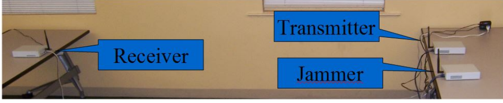
Figure 6.5: In this figure, we show the SDR setup we used for testing the STIR-jamming algorithms.
